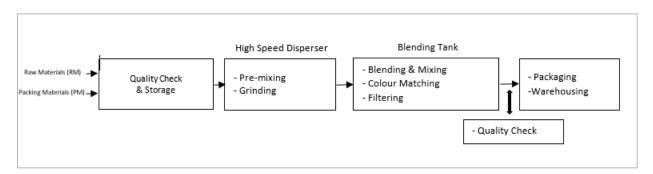
*Inspection of Raw Materials:* Upon delivery, the incoming materials are inspected pursuant to quality control specifications. Raw materials are accepted and stored only after they have passed the relevant quality control tests. Bulk liquid raw materials that have passed the quality control tests are transported from tanker-vehicles and loaded and pumped onto on-site storage vessels.
